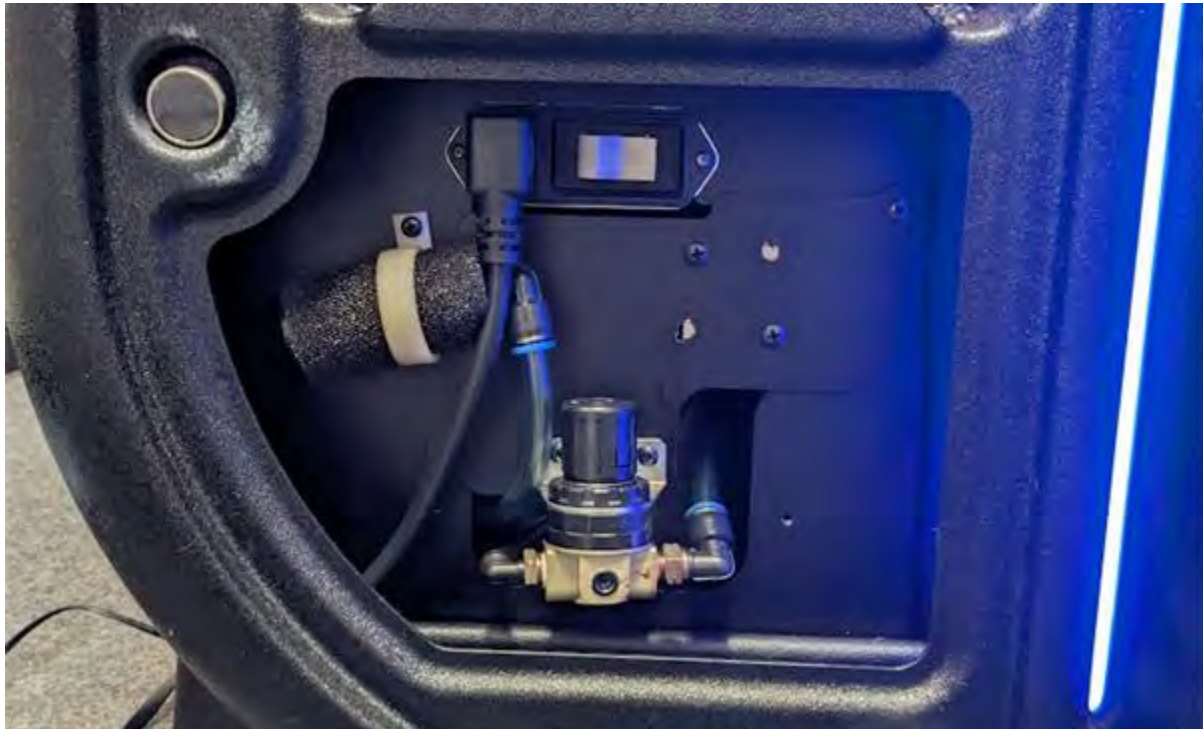
[Booth power switch, compressor filter and air regulator]
