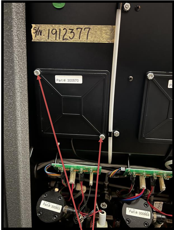
11/32in nuts securing RFID antenna
